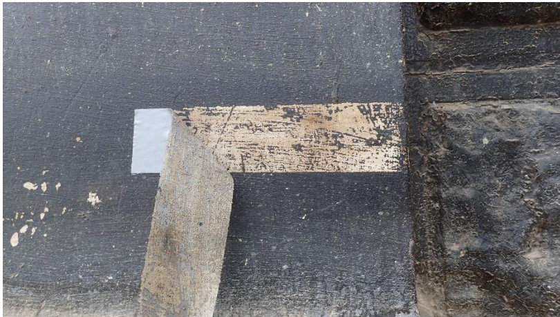
Figure 5. Black waterproof coating removed with duct tape.
