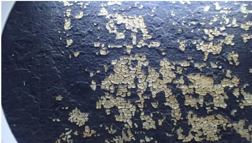
Figure 4. Paint layers under black coating.
