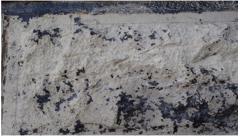
Figure 19. Detail of Trial 19 showing erosion of surface.
