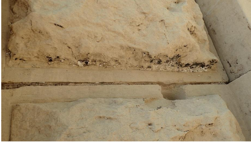
Figure 23. Prosoco Limestone Restorer, Reclaim, and Afterwash: coatings remain on underside.
