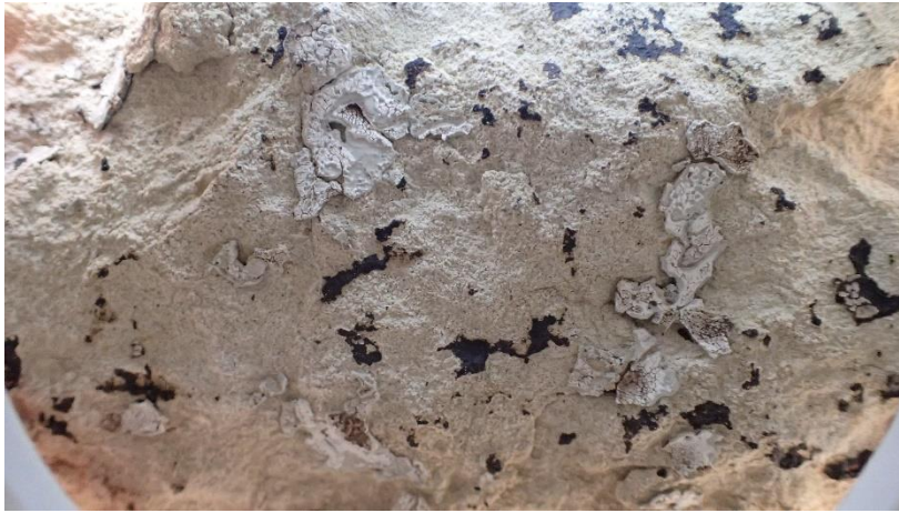
Figure 13. Photomicrograph of Trial 8 with paint residue in pores.
