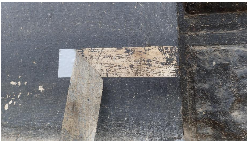
Figure 5. Black waterproof coating removed with duct tape.
