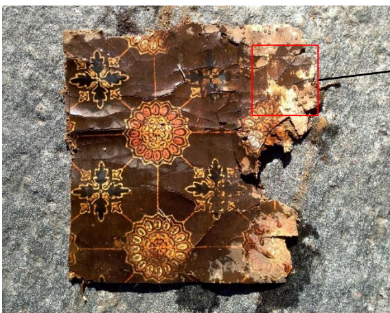
(left) This is a more elaborate design of Kamptulicon I found while researching the product. The paint is applied over the cork and India rubber mixture. The whole of the product is applied over a fabric backing (above, arrow)
