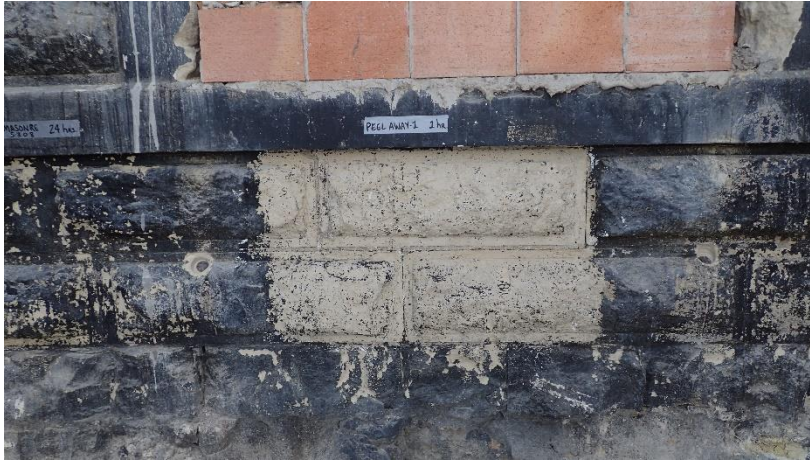
Figure 11. Dumond PeelAway 1 and Neutralizer: Trial 8.
