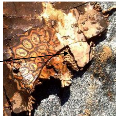
(left) This is a more elaborate design of Kamptulicon I found while researching the product. The paint is applied over the cork and India rubber mixture. The whole of the product is applied over a fabric backing (above, arrow)
